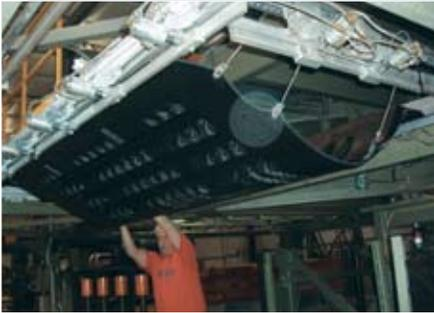
After cooling, the formed composite inner panel is removed from the clamping frame. The part will be trimmed prior to bonding to the outer skin.
