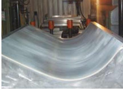
The aluminum vacuum forming mold for the Class A thermoplastic olefin (TPO) outer skin. As with the inner panel, cooling lines are cast into the mold to remove heat from the preheated sheet.
