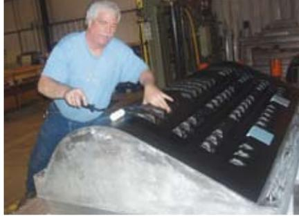
A technician applies adhesion-promoting liquid primer to the bonding surfaces of the composite inner panel. The primer also is applied to the inside of the outer skin panel.
