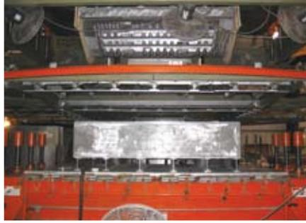
Preheated, lofted sheet is placed between the aluminum upper forming tool and the mating lower tool. The mold is closed under low pressure and the sheet is cooled.
