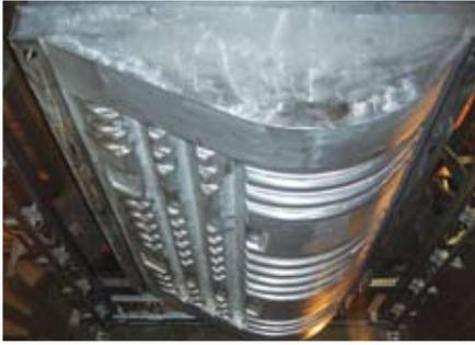
Detailed aluminum forming tool for the lofted glass-reinforced polypropylene structural inner panel. Cooling lines are cast into the mold to remove heat from the preheated sheet.
