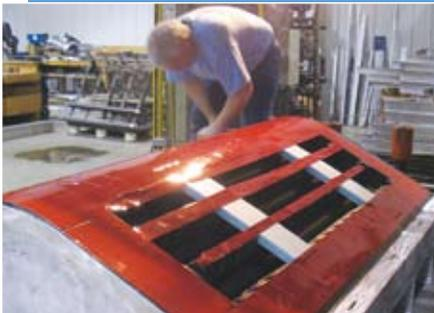
Foam tape adhesive is applied to the bonding surfaces of the inner panel. The outer and inner panel are mated at low pressure to insure full contact.
