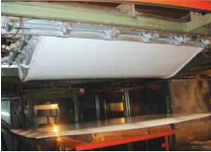
The formed outer TPO skin has been indexed to the removal station and is ready to be unloaded from the clamping frame and trimmed.
