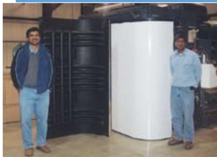
Two finished doors, after robotic trimming (the one at left is viewed from the inside, the one at right, shows the outside surface).
